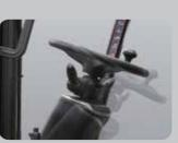
Adjustable steering wheel To achieve a comfortable drive position, the angle of the steering column can easily be adjusted through a lever on the right-hand side of the steering column.
