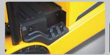
Low entrance height In order to get in and out of the cabine in an easy and safe way the height of the entrance step is only 400mm high.
