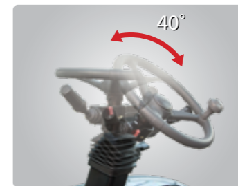
Adjustable Steering Column
